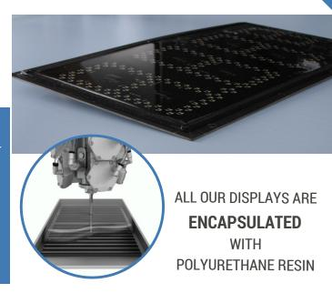
RESIN ENCAPSULATION PROTECTS AND INSULATES THE ELECTRONIC COMPONENTS FROM **HARSH ENVIRONMENTS**, MOISTURE, VIBRATION, HUMIDITY AND CHEMICALS.
